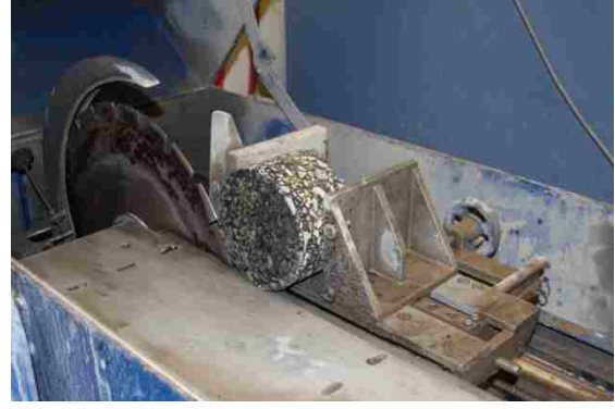
b) Sample cutting in the laboratory
