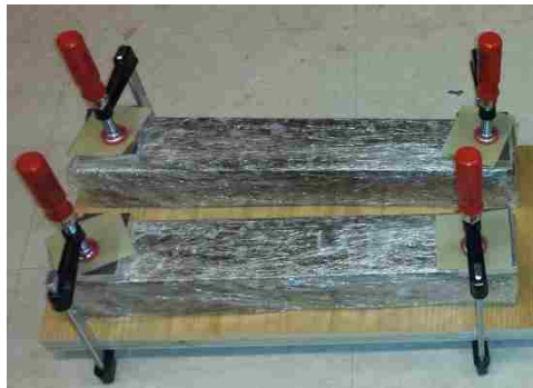
c) Restraining the samples with wood
