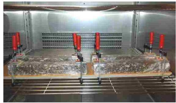
d) Applying cyclic temperature
