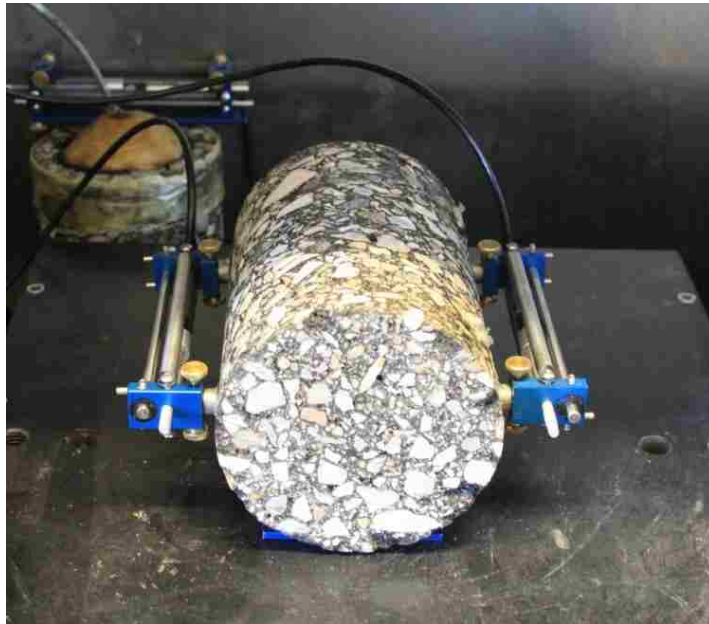
Figure 14. Measuring the thermal expansion-contraction (Vertical Direction)
